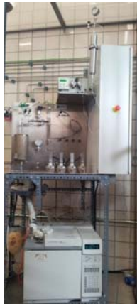
High pressure fixed-bed lab reactor
